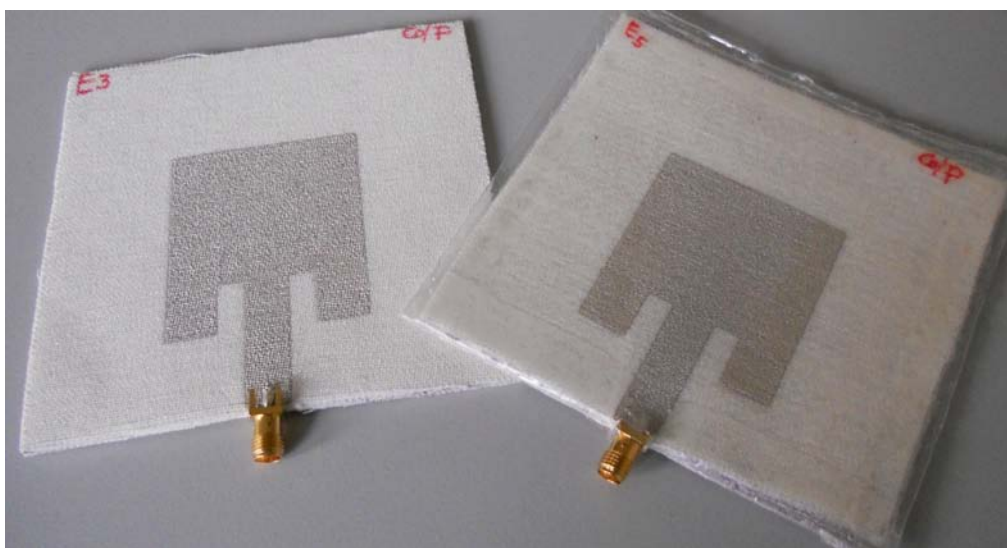
Figure 3. Printed antennas with conductive ink; left is an uncoated and right a coated antenna
