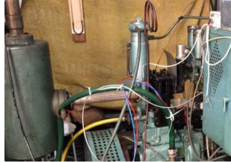
Fig. 2. CFR Octane Rating Unit Engine equipped with LASER spark plug
