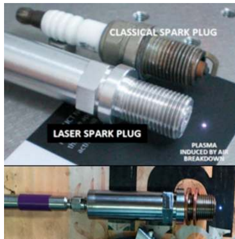
Fig. 3. A photo of a LASER spark plug is shown in comparison with a classical spark plug. The plasma induced in air by optical breakdown is visible. (Courtesy of INFLPR, Laboratory of Solid-State Quantum Electronics, Magurele, Romania)
