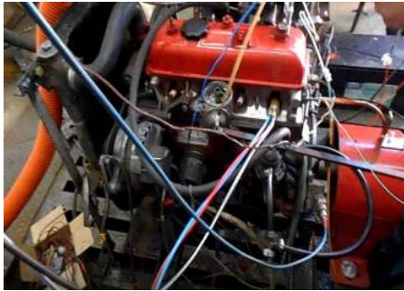
Fig. 1. Dacia Single Cylinder SI Engine equipped with LASER spark plug
