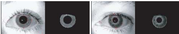
Fig. 5. Example of images of the BioSec database with the annotated circles modeling iris boundaries and eyelids.
