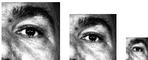
Figure 2.32: A comparison of down-sampled images and their pixel counts. From left to right: Un-deteriorated Image (80,089), down-sampled to 80% (64,071), down-sampled to 40% (32,035).
