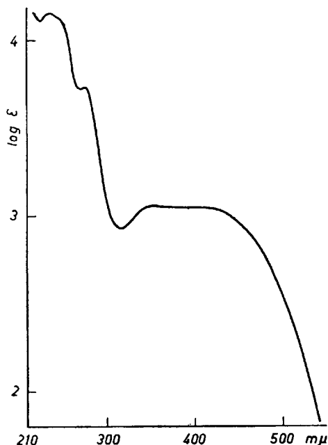
Fig. 3. Light absorption of (2-hydroxyphenyl)- p -benzoquinone (XXII). Solvent: 95 % ethanol.
