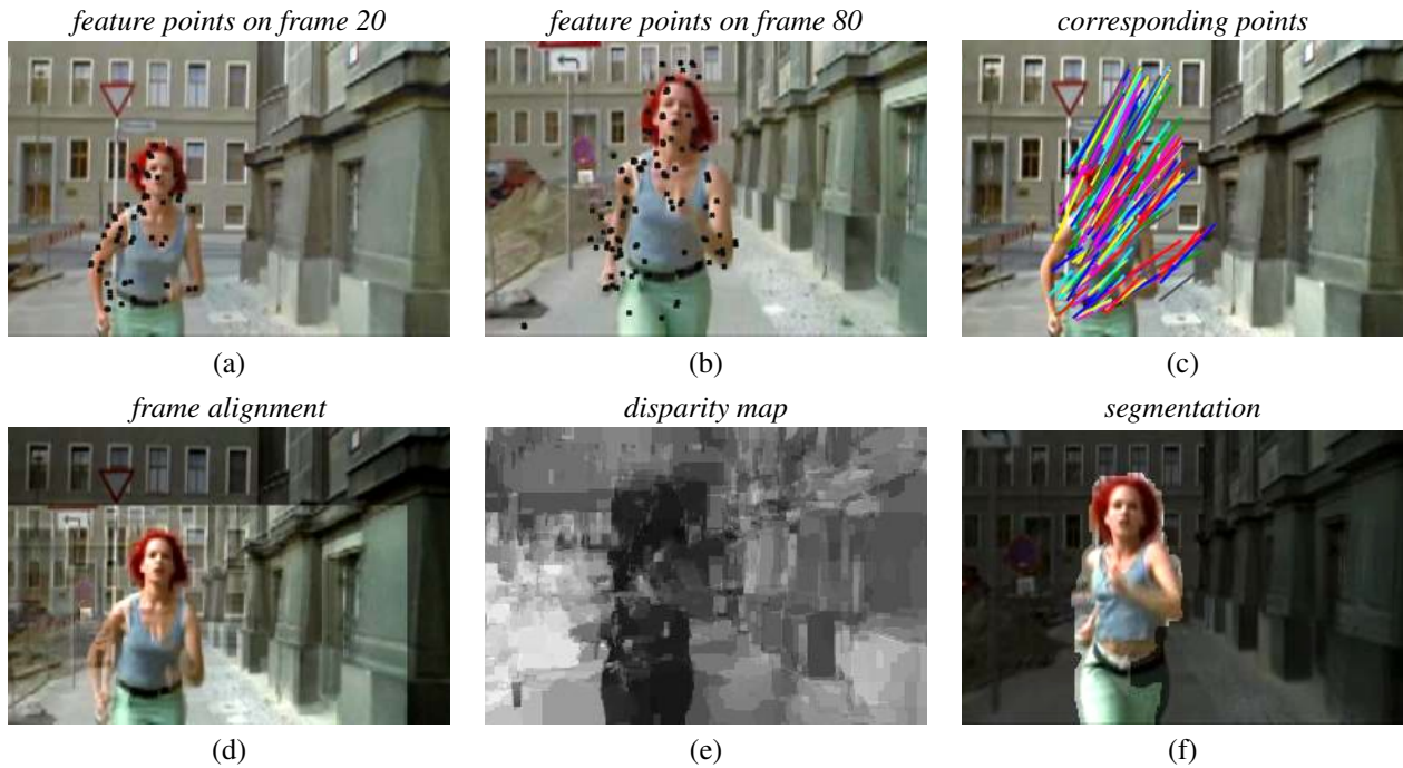
Figure 5. Matching, alignment and segmentation of periodic motion. (a)-(b): Two periodic views selected from the same video sequence and separated in time by three values of a period. Black dots show locations of detected WLSTF points for each frame. (c): Matches of WLSTF points in (a)-(b) that are consistent with the estimated dynamic homography \hat{H}_{per} . (d): Result of alignment of the frame (b) to the frame (a). The sum of the frame (a) and the transformed frame (b) is shown. (e): Estimated disparity map with low values corresponding to regions with good alignment of periodic frames. (f): Final result of segmentation.
