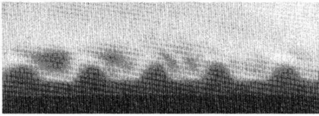
Fig. 10. An 0.411- \mu\text{m} grating ion-etched into GaAs through a photoresist mask.
