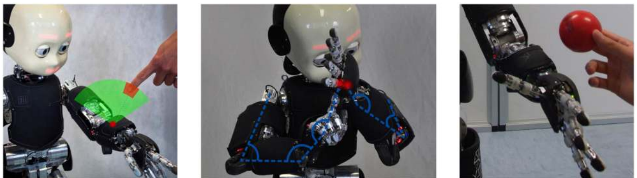
Fig 1. Illustration of the setup of different scenarios. (left) Receptive field above one of the left forearm taxels. (middle) iCub double-touch behavior with a simplified schematic of the kinematics and joint angles. (right) An object approaching the left forearm.
