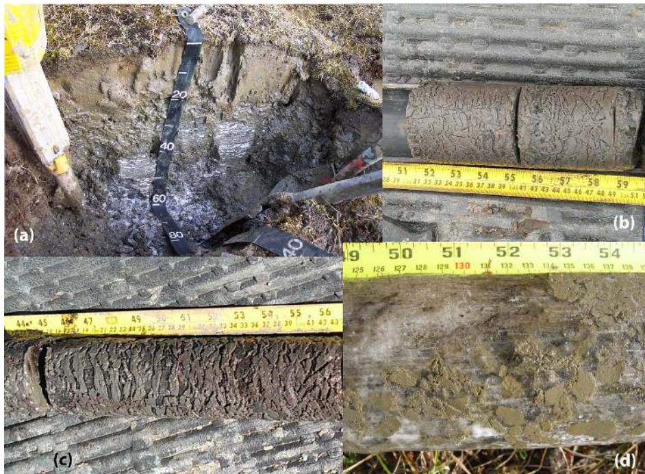
Figure 1. Examples of common cryostructures: (a) lenticular structures visible below 30–40 cm in a freshly exposed profile of an earth hummock, Mould Bay, Arctic Canada (reprinted by permission, ASA, CSSA, SSSA); (b) lenticular structures transition to a reticulate structure at 130–150 cm in a core extracted from the center of a low-centered ice-wedge polygon; (c) lenticular structure; and (d) suspended (ataxitic) structure.
