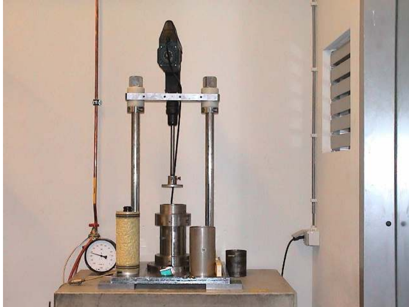
Figure 4.8 Kango hammer and an aggregate skeleton specimen
