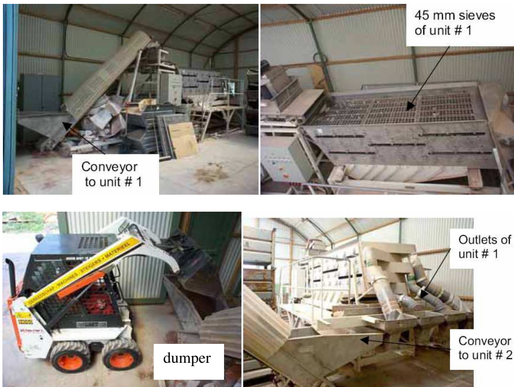
Figure 3.2 Large scale sieving equipment and the dumper (Van Nierkerk 2002)
