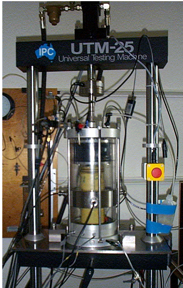
Figure 4.1 UTM 25 triaxial cell
