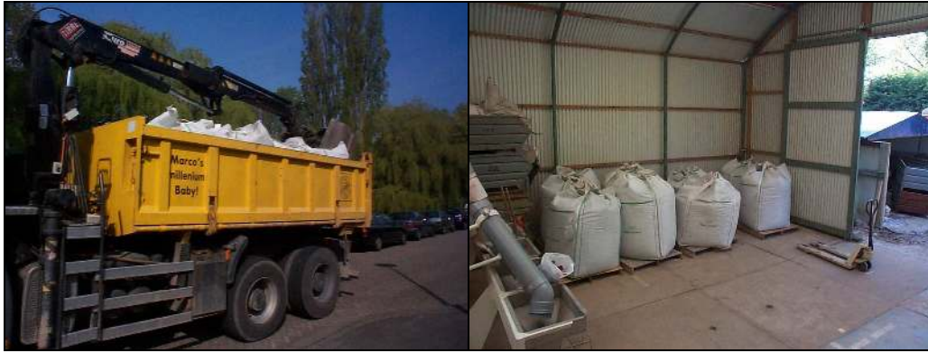
Figure 3.1 Delivery of the aggregates and the aggregate storage area
