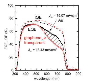
**Figure 3.** External (EQE) and internal quantum efficiency (IQE) spectra. The open red circles and full black squares correspond to the measured EQE of the graphene and Au contact, respectively. The red and black dashed lines correspond to the calculated IQE for graphene and Au contacts, respectively. The devices were illuminated from the glass/SnO<sub>2</sub>:F side.
