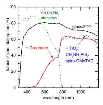
Figure 4. Transmission spectra of glass/SnO<sub>2</sub>:F (solid black line), the perovskite top solar cell layer stack glass/SnO<sub>2</sub>:F/TiO<sub>2</sub>/CH<sub>3</sub>NH<sub>3</sub>PbI<sub>3</sub>/spiro-OMeTAD (dotted blue line), and of glass/SnO<sub>2</sub>:F/TiO<sub>2</sub>/CH<sub>3</sub>NH<sub>3</sub>PbI<sub>3</sub>/spiro-OMeTAD/graphene/support (solid red line). Absorption of CH<sub>3</sub>NH<sub>3</sub>PbI<sub>3</sub> on glass (dotted olive line).
