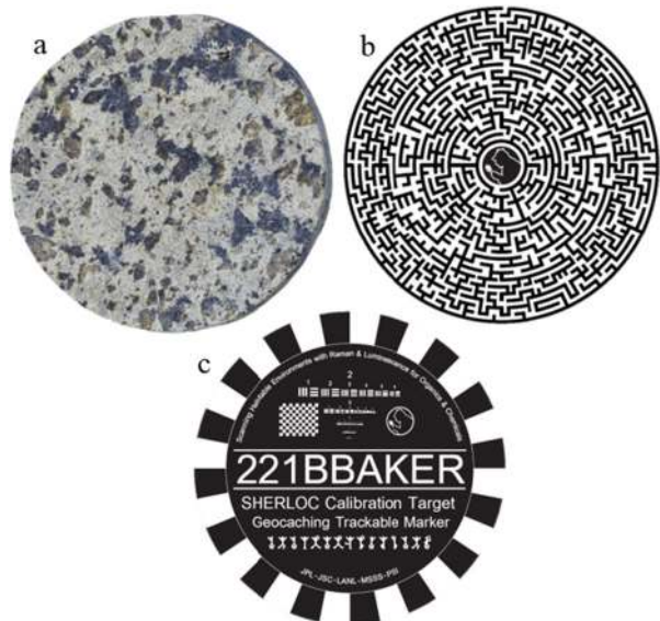
Fig. 28 Photograph of SHERLOC Calibration Targets (from the FM). (a) #3 Mars Meteorite, (b) #4 Intensity Target Maze, and (c) #6b Geocaching Trackable Marker coin
