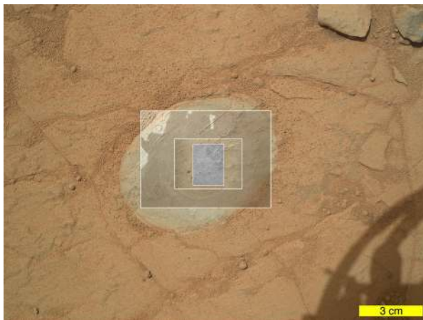
Fig. 67 Example series of nested ACI and WATSON images at typical working distances anticipated for the Perseverance mission: a 10.1 \mu\text{m}/\text{pixel} grayscale ACI image, nested within a 2.7 cm working distance WATSON image, nested within a 6.8 cm working distance WATSON image, nested within a 26.4 cm WATSON context image. This nested suite was simulated using MSL MAHLI images from Sol 150 of a mudstone target named Ekwir-1. The nested position of the ACI may be rotated differently than shown here, relative to the WATSON data, unless the turret is positioned in a manner that accounts for the natural 20^\circ rotation of the different CCD's (example in Fig. 52)
