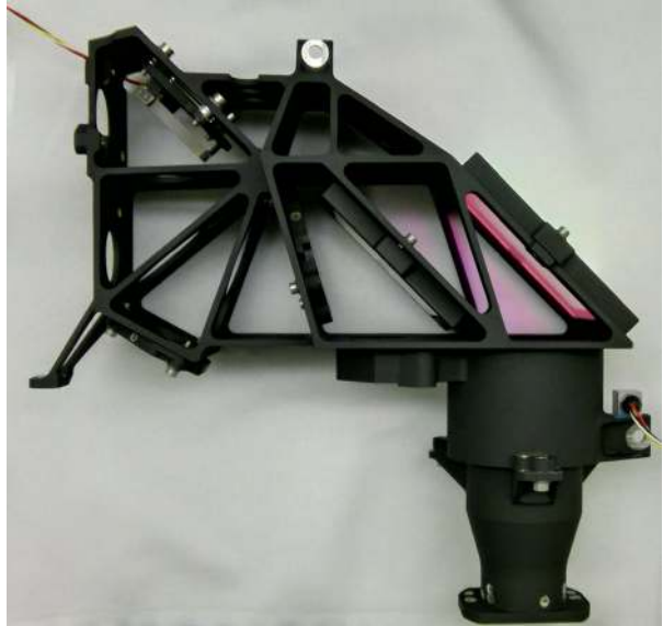
Fig. 34 The foreoptics of the SHERLOC optical bench
