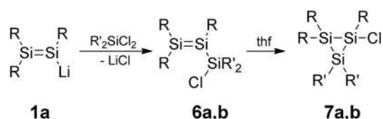
Scheme 3. Synthesis of \alpha -chlorosilyldisilenes 6a,b and cyclotrisilanes 7a,b ( R = \text{Tip} ; 6a , 7a : R' = \text{Me} ; 6b , 7b : R' = \text{Ph} ). [12]
