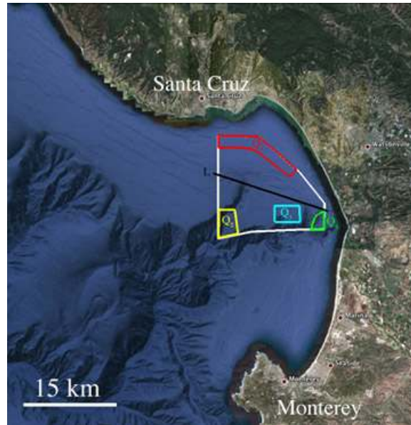
Figure 11: The white polygon delineates the general survey Region Q_1 and the colored polygons designate the high-interest regions used as input to our mission planning algorithms. Region Q_1 (red) is the LATMIX region, Region Q_2 (yellow) is an area near an MBARI mooring buoy, Region Q_3 (cyan) was an area with an active algal bloom, and Region Q_4 (green) is an area near a river mouth.
