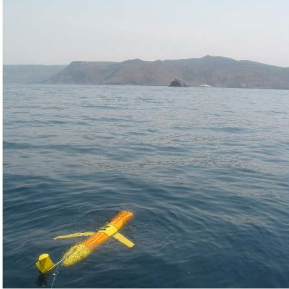
Figure 3: One of two Slocum gliders owned and operated by the USC Center for Integrated Networked Aquatic PlatformS (CINAPS) (Smith et al., 2010b) preparing to start a mission off the Northeast coast of Santa Catalina Island, CA.
