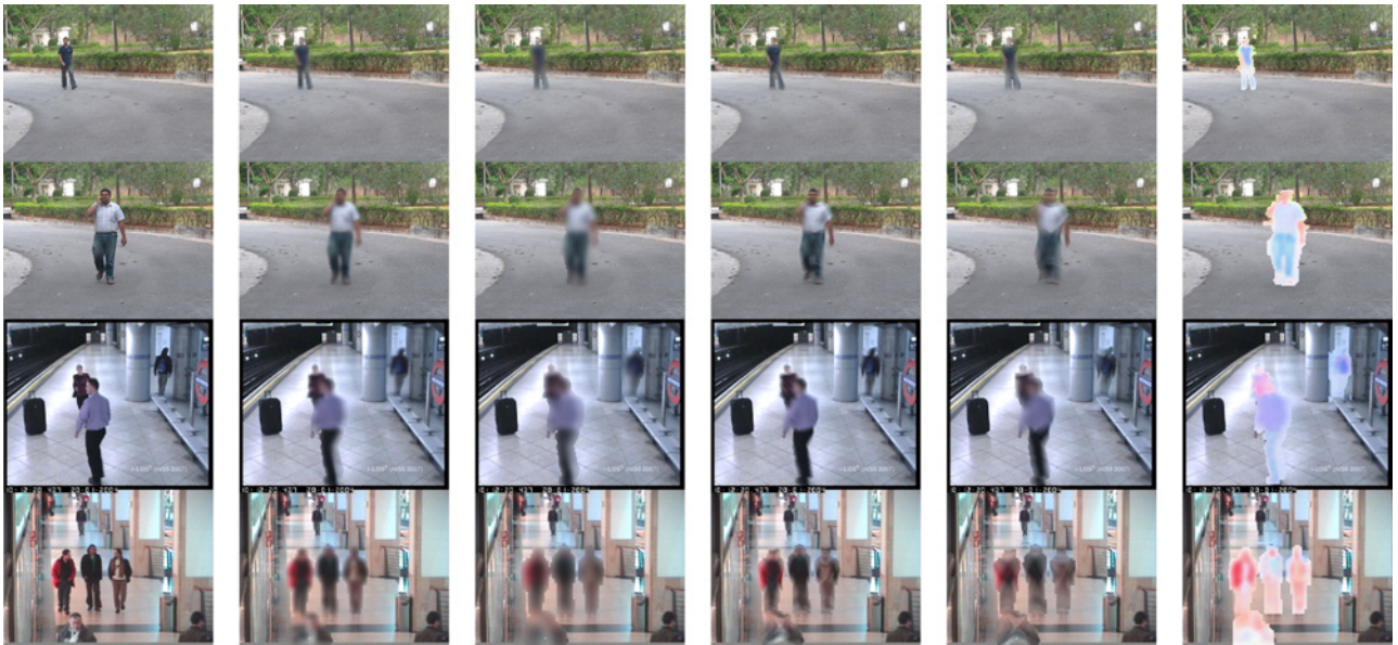
Fig. 3. First column shows the clear frame. The next five columns show the output of Blur-2, Blur-4, LIC-10, LIC-20, and Blur-2 followed by an intensity space compression, in that order.
