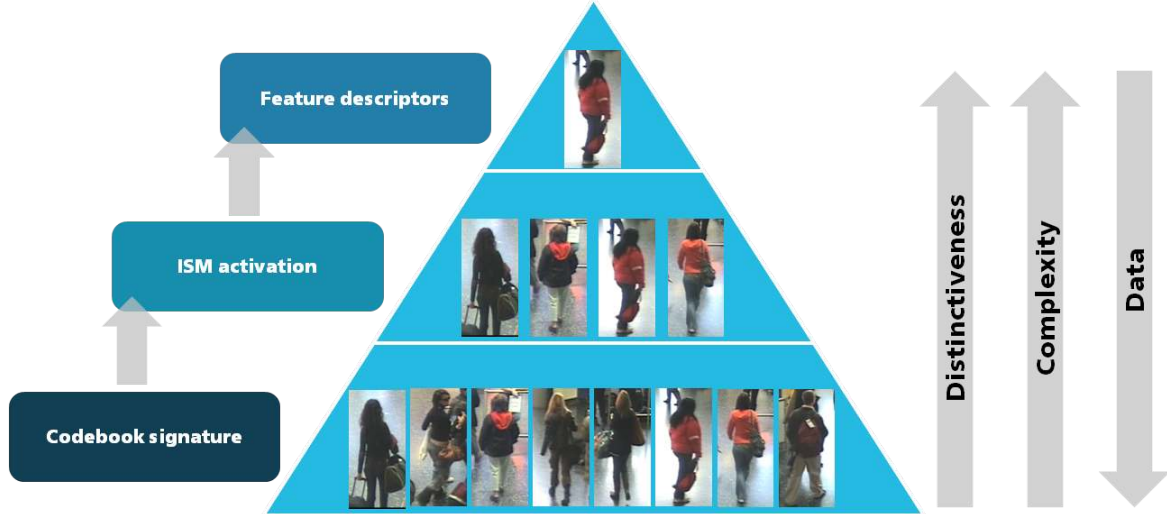
Figure 3. Overview of the 3-staged re-identification approach. In stage 1, the codebook signatures (activation signatures) are compared. Second stage uses ISM activation by adding spatial feature distribution. Third stage compares the high dimensional SIFT descriptors. By using the stages in a cascade amount of persons that have to be considered can be reduced in each stage. Thus, in the computational most expensive stage 3 which provides the highest distinctiveness, only few database models have to be considered for a query model.
