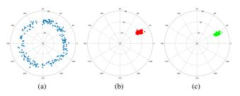
Fig. 3: CSI extracted phase processing example. In (a), (b), and (c), the raw, sanitized and median filtered phases of a single subcarrier, respectively.
