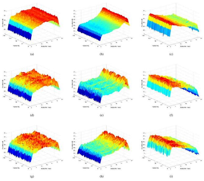
Fig. 5: Heatmaps M-derived 3D surfaces examples for 200-packets acquisitions in the three rooms, i.e., a hallway, office, and conference hall, in the first, second and third row, respectively. Images (a), (d), and (g), correspond to no obstacles between TX and RX APs; while triples (b), (e), (h) and (c), (f), (i) show two different persons of the collected dataset.
