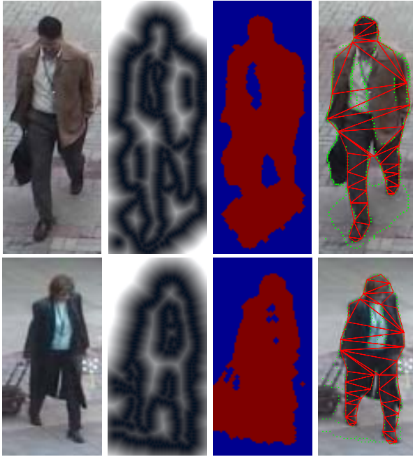
Figure 4. This figure illustrates two examples of fitting the decomposable triangulated model to individuals. The cropped image, edge feature image, foreground mask, and fitting results are shown from left to right. The green dots show the candidate locations for the model points. Observe that the model fits well to the individuals despite the presence of bags, shadows, additional interior edges due to different clothing etc.
