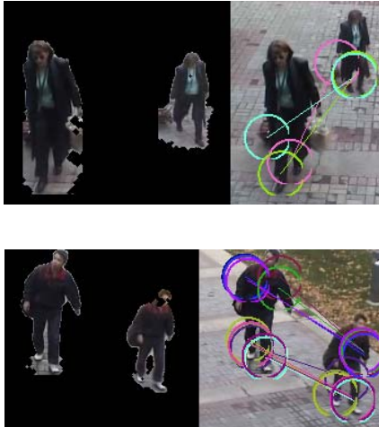
Figure 2. Two examples of the interest operator matching algorithm. On the left are two images that are to be compared. On the right are the identified correspondences and associated signature regions.
