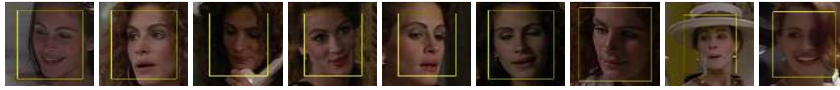
Fig. 1. Example face detections of the Julia Roberts’ character in the movie ‘Pretty Woman’. Note that detections are not always perfectly frontal. Note also successful detections despite varying lighting conditions, changing facial expressions and partial occlusions.
