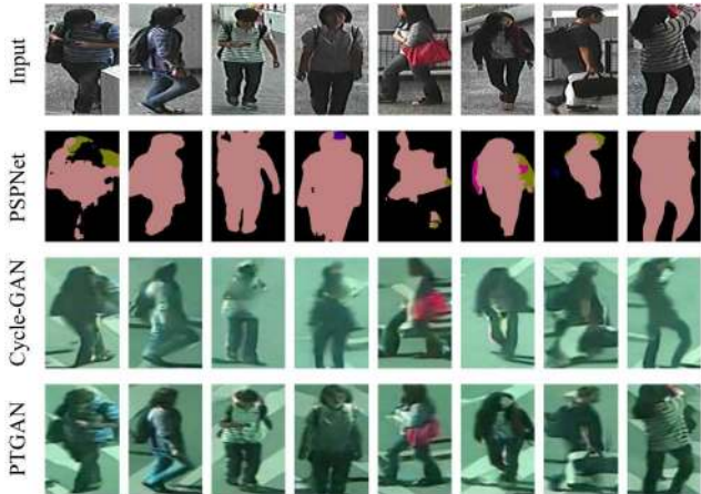
Figure 4: Comparison of the transferred images by PTGAN and Cycle-GAN from CUHK03 to PRID-cam1 . The second row shows the segmentation results by PSPNet. The pink regions are segmented as person body regions.
