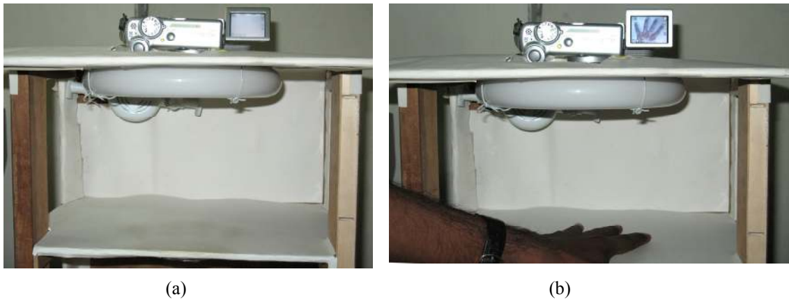
Figure 2: Image acquisition setup in (a) and acquisition of a sample finger back image in (b)
