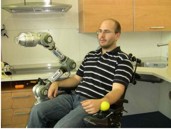
Fig. 3. ASIBOT assistive robot that is fixed on a wheelchair’s installed DS.
