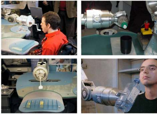
Fig. 7. ASIBOT can use a variety of tools that are adapted to user's needs.
