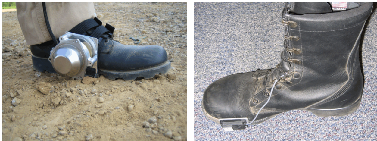
Fig. 1: The University of Michigan’s two IMUs mounted on rescuer’s boots. (a) The SiIMU used in our earlier proof-of-concept prototype; (b) the small-sized nIMU, described in this paper.
