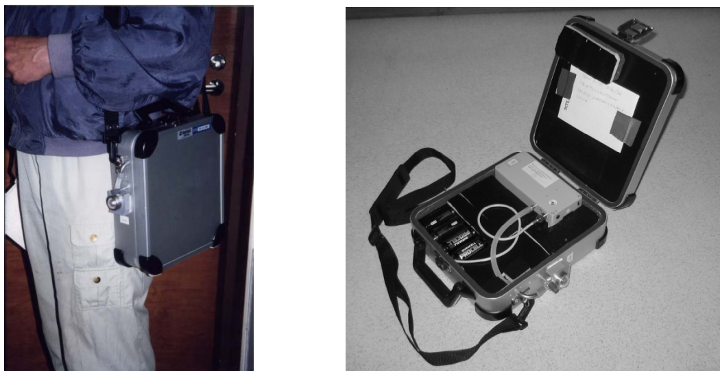
Fig. 5. The personal exposure monitor (PEM), with the button sampler.
