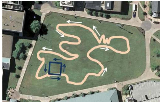
Fig. 13. Procedure for loop-closing half-hour walks. 1) Short walk around a square (11.7 m/edge) for 5 min. 2) Longer half-hour walks around the same square as a short walk or a random path (paths are shown for illustrative purposes only).
