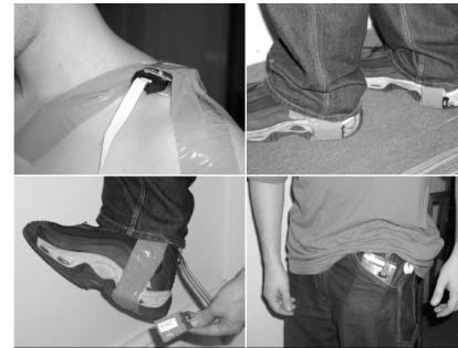
Figure 7. Clockwise from top left: compass sensor taped to shoulder; accelerometer sensors attached to pedestrian's shoes; Bitsy motherboard carried in pocket; and accelerometer sensor, extracted from sole holster to show size.
