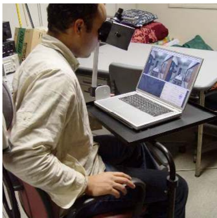
Figure 8: Stereoscopic display of QTVR imagery. A nomadic version, “μVR 4 U 2 C,” platformed on the Sharp SH25liS, provides an autostereoscopic equivalent for mobile phones.
