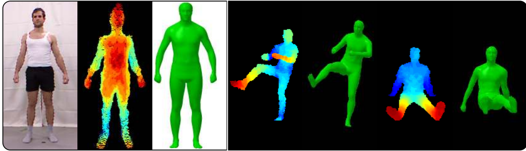
Figure 1. (From left to right): Actor standing in the front of a single Kinect camera. Color coded depth data (red is near, blue is far) as obtained from the Kinect. Automatically estimated body shape of the actor. Two complex poses reliably tracked with our algorithm (left: input depth, right: estimated pose).
