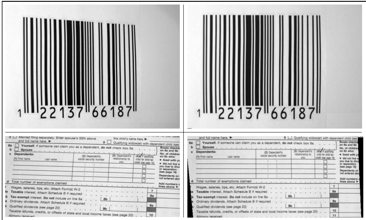
Figure 5. Identification of Vanishing Points Robustly Leads to Rectification. Many of our document images have enough clues for identification of vanishing lines in the form of parallel and perpendicular lines.
