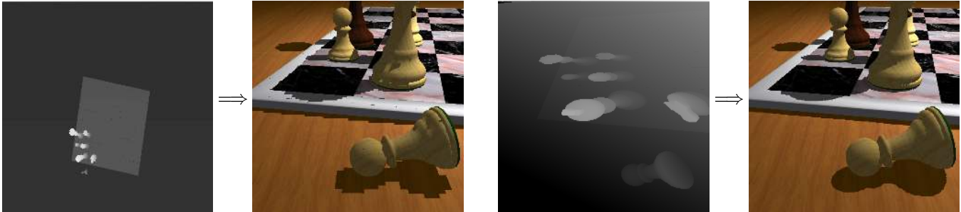
Figure 1: (Left) Uniform 512x512 shadow map and resulting image. (Right) The same with a perspective shadow map of the same size.
