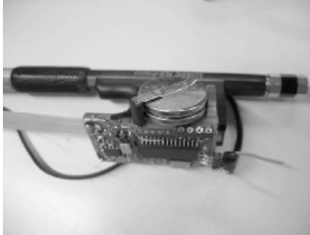
Figure 1: Module placed at the frog of the violin bow to measure players' bowing movements. It consists of two accelerometers and a RF transmitter, powered with batteries.
