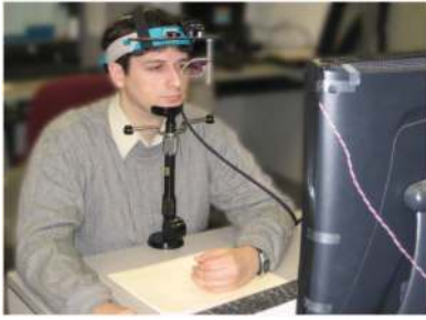
Fig. 5. Our experimental setup for the user study with the ISCAN ETL-500 eye tracker.
