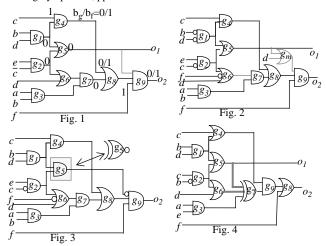
Let  $g_s$  has mandatory assignment 0,  $g_d$  is a dominator (AND gate) and  $g_I$  is a fault propagating wire.
