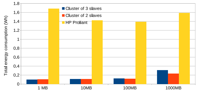
Fig. 4: Total energy consumption the Mandelbrot set task on a smartphone cluster and a server.
