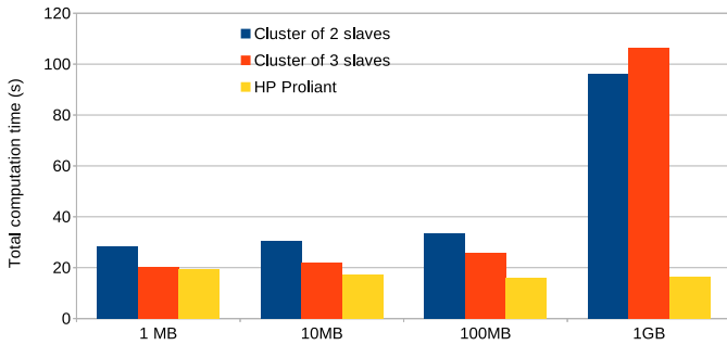
Fig. 3: Execution speed of the Mandelbrot set task on a smartphone cluster and a server.
