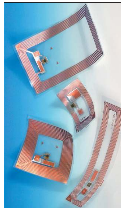
Figure 2. Texas Instruments TagIt passive RFID tags have onboard read/write memories. These tags are delivered in a polymer substrate in reels for easy handling. They are so cheap that they are disposable and truly pervasive. (photo courtesy of Texas Instruments)
