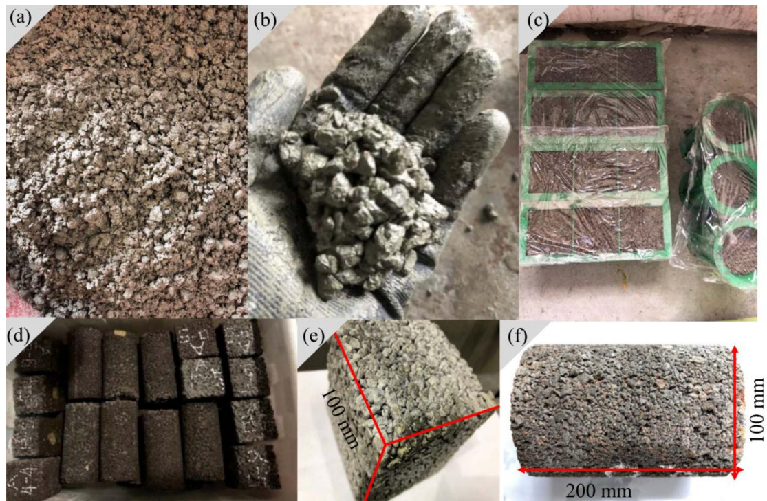
232 233 Figure 3 The fabrication processes of pervious concrete: (a) wet status of pervious concrete, (b) 234 manual examination in hand, (c) casting of fresh pervious concrete in cubic and cylinder moulds, 235 (d) pervious concrete specimens stored in a chamber, and illustration of selected (e) cubic and (f) 236 cylindrical specimens.
