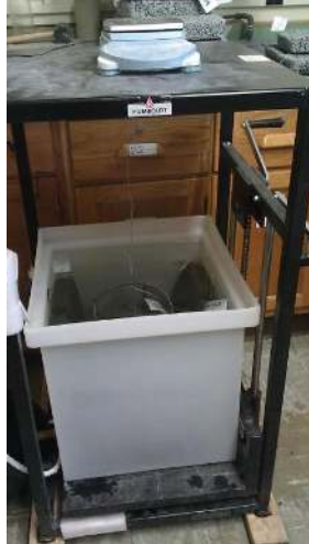
Figure 3.1: Pervious concrete samples submerged underwater during porosity test
