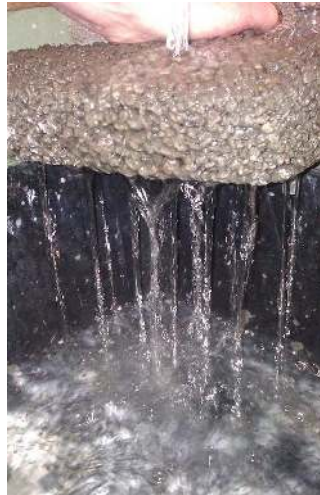
Figure 3.2: Water infiltrating completely through a pervious concrete sample
