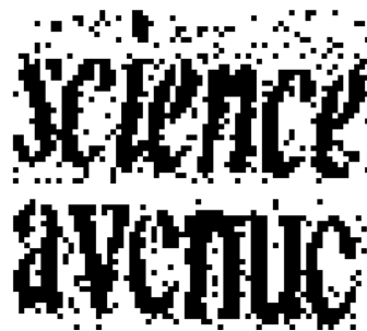
Figure 2. Examples of synthetically generated images of printed words which are machine-illegible due to degradation parameter thrs = 0.02.
