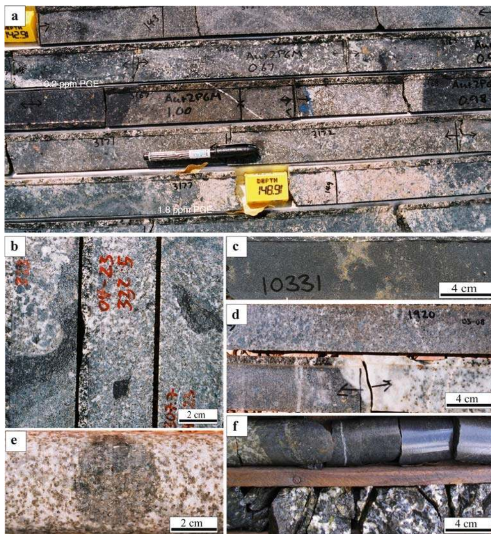
Fig. 5 Lithologies of the LMF and MANO on Rooipoort and Moordrift. a Varied-textured gabbronorite, showing variable grain size and color index, interlayered with decimeter-wide chromitite seams and felsic veins. Borehole 03–12, upper portion of LMF. b Schlieren and clasts of chromitite in gabbronorite, central-upper portion of LMF, borehole 04–23. c Massive chromitite enriched in sulfide, central portion of LMF, borehole 04–22. d Melagabbro-norite containing weak PGE enrichment overlying anorthosite and leucogabbro-norite. Central portion of MANO, borehole 03–08. e Boulder-like aggregate of melagabbro-norite, upper portion of MANO, borehole 03–08. f UG-like chromitite within gabbro-norite on Moordrift, borehole MD4, 895.4–896 m
