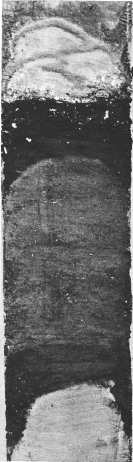
Figure 4. Characteristic sequences of the Upper Sapropel of the Hellenic Trough (128-3-5, 35 to 13 cm). The first sequence starts with a black foraminiferal-quartzose clayey sand which grades upward into a marl ooze of lighter color. The second sequence is reduced to the basal layer of dark sand. It is overlain by a new sapropelitic sequence which starts by a cross-bedded white foraminiferal sand.
