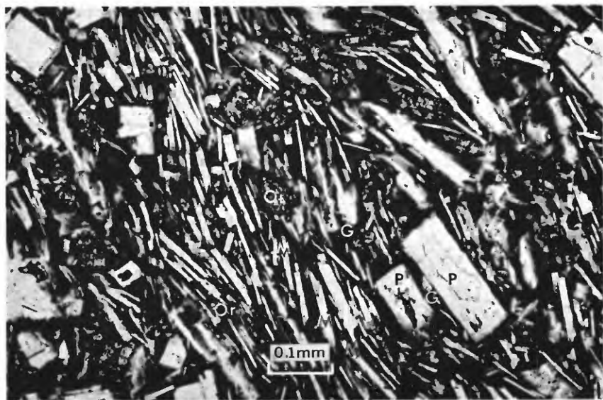
FIGURE 17.—Intersertal-trachytic texture in intrusive andesite. Euhedral plagioclase microphenocrysts (P) and elongate microlites (M) separated by brown glass (G). Orthopyroxene (Or) grains partly in intergranular position. Plane light, \times 120 . Sample MJW-10.
