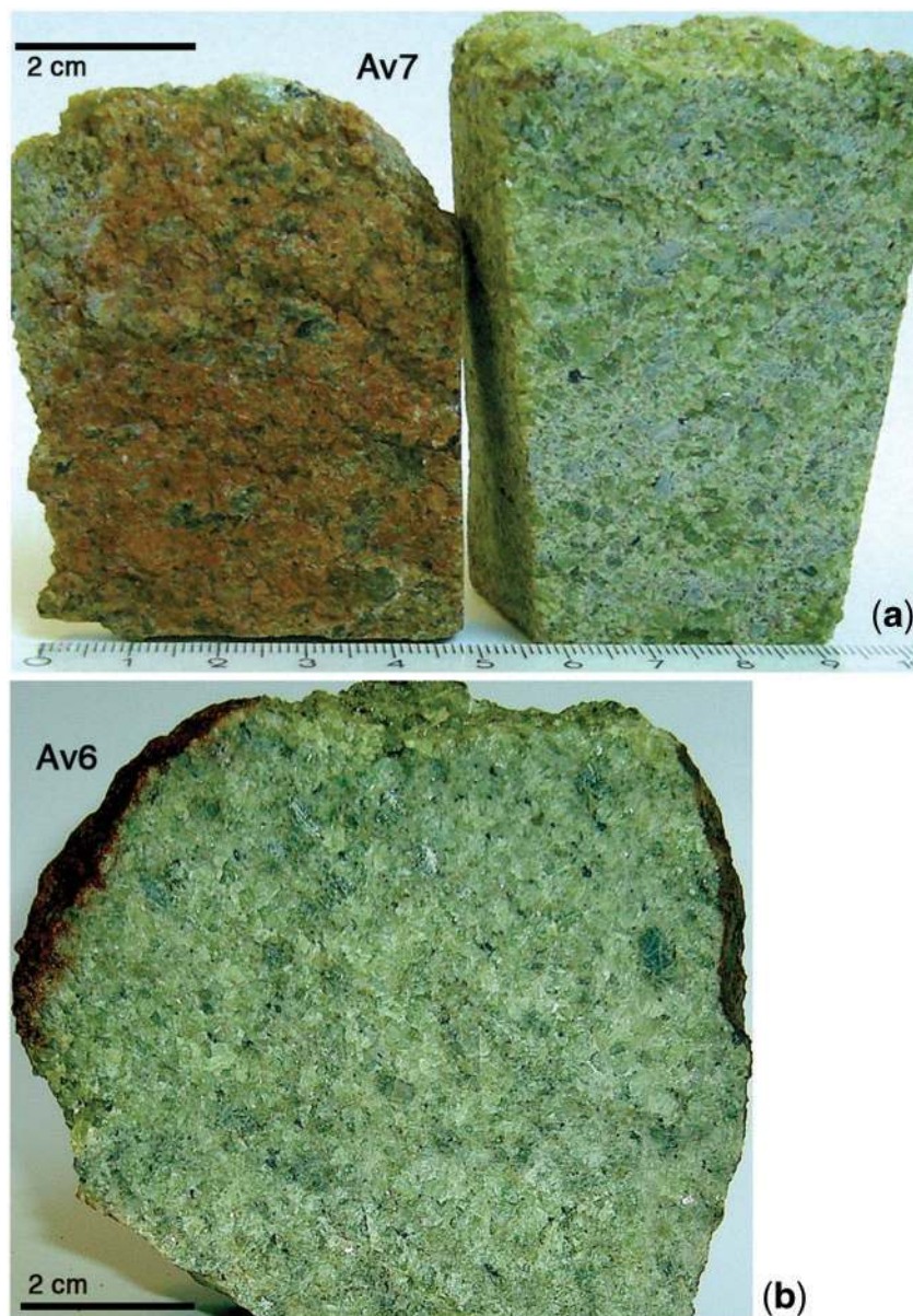
Fig. 2. Photographs of sawn hand specimens of peridotite xenoliths from the Avacha volcano. (a) Oxidized alteration crust (left) of xenolith Av7 removed to obtain alteration-free material (right) to make bulk-rock powder. (b) Xenolith Av6 has altered crust (upper left) and amphibole-rich selvages (upper right) outside but shows no apparent veining or alteration products in the centre.
