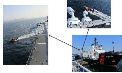
Figure 3. IPATCH cameras were positioned on a tower located at the stern of the Partisan Vessel.
