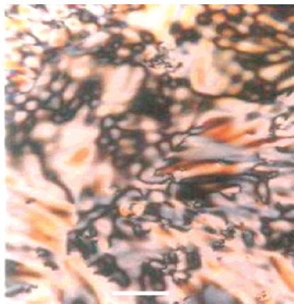
Figure 13. Typical threadlike texture of the nematic (N) phase. \alpha = 1.85 , \phi_s = 40 , T = 30 °C. Scale bar represents 0.1 mm.
