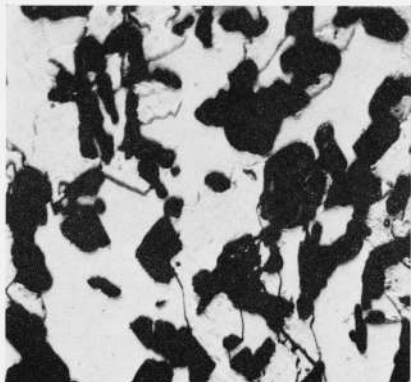
FIGURE 8. Substructure in the \gamma phase. Alloy 70 Fe-26 Mo-4 Ni after reheating to 2,000° F for 75 hours.
