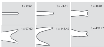
FIG. 6. Irregular tip splitting scenario. We used D/\xi v_R = 1.85 and \Delta = 3.6 ; the system size is 600 \times 400 . Time is given in units D/v_R^2 . Minor numerical noise breaks the symmetry of the competing sidebranches.
