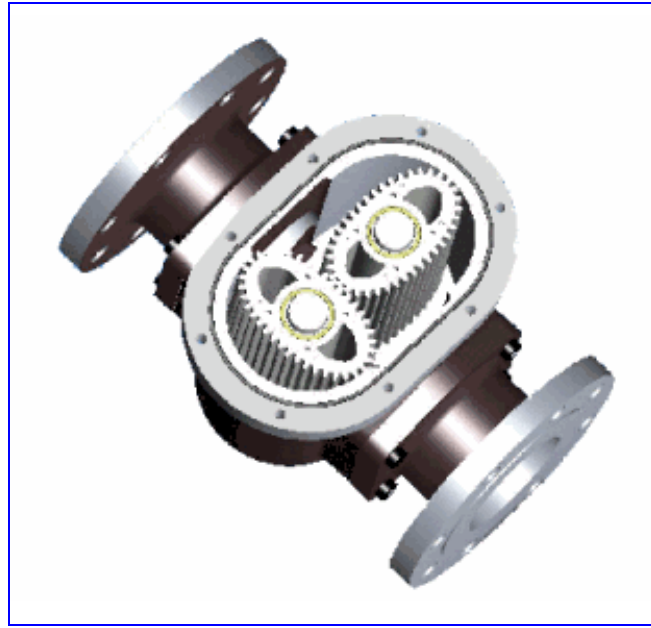
Figure 2.9 Chambers in positive displacement meter (Yeung, 2003)
