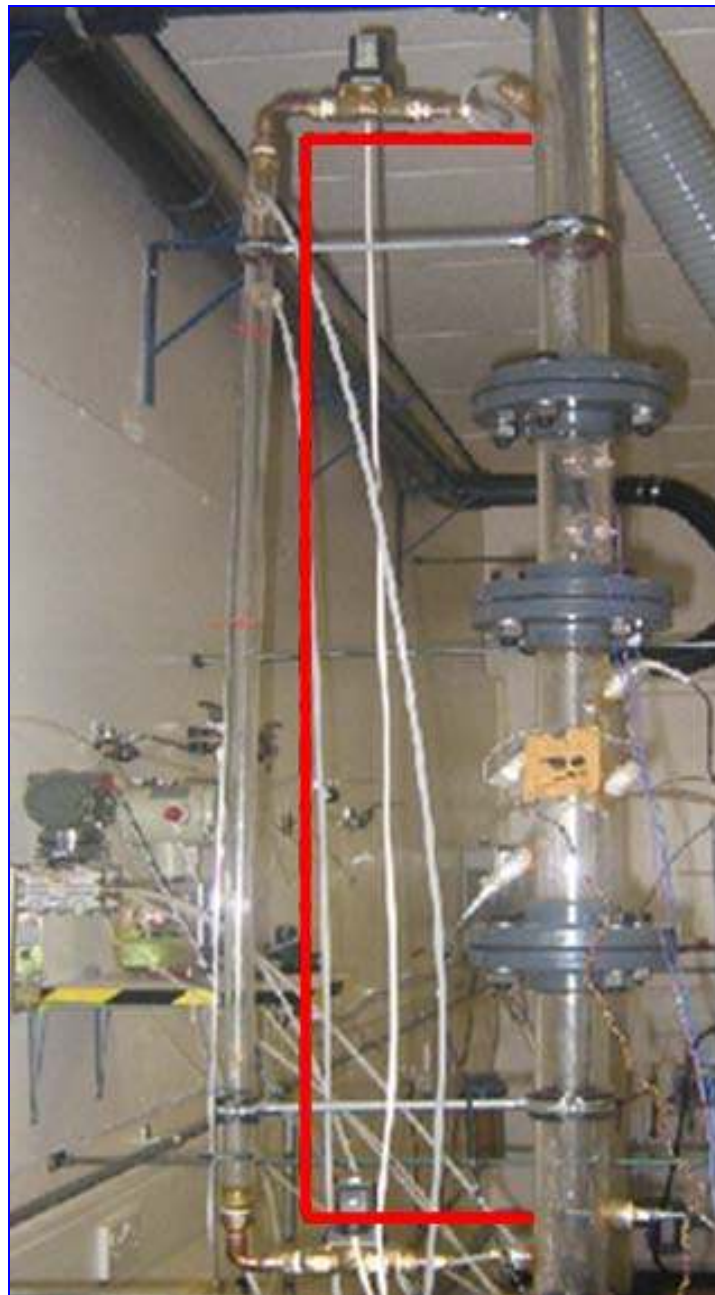
Figure 4.1 Sensor tube, to the left and outside the red line
