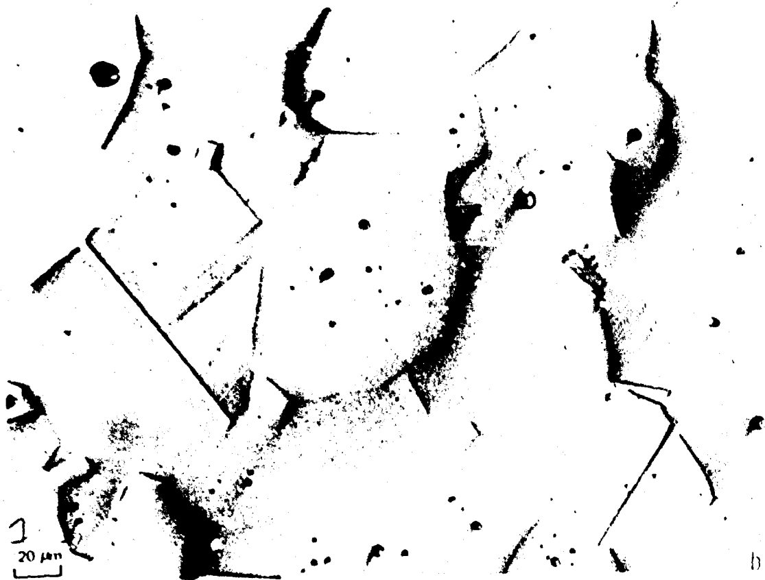
Figure 6. Microstructures of single-phase cubic aluminum oxynitride spinel; T = 1975 C; 30 mole % AlN; 1 hour.
