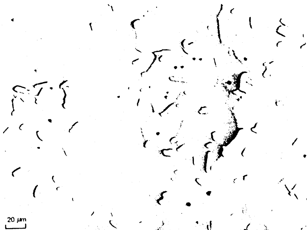
a. 2025 C - in Liquid + ALON(SS) Field; 10.04 Wt% Loss
