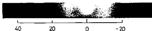
Figure 2. Scattering pattern from the blend of 39.5 wt% PS at a quench depth \Delta T = 3.7^\circ\text{C} and a time t = 50 min after quenching.
