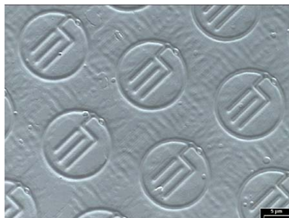
Fig. 3a. Logo array fabricated by laser MLA lithography.
